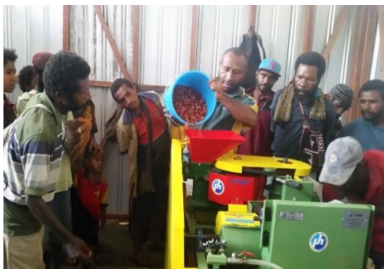
Plate 2: Farm trial using a demucilager
