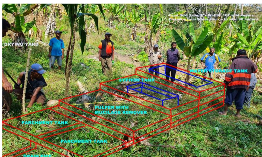
Plate 4: Site sketch for the establishment of a demucilager in a CBB environment.
