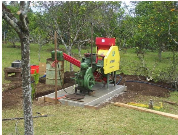
Plate 1. Demucilager used to remove pulp and mucilage from coffee cherry.
